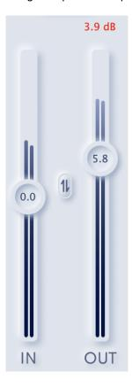
Units are displayed in dB scale. If the signal peak is greater than 0dB, the warning (digits in red color) will pop out on the top of the fader. Click the digits can let it disappear. If the plugin is overdriven by excessive input volume, the signals will be gradually colored, therefore having more analog distortion.
