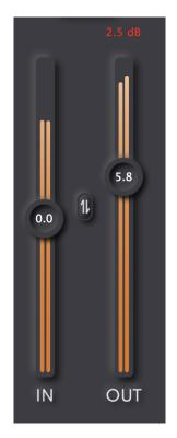
Units are displayed in dB scale. If the signal peak is greater than 0dB, the warning (digits in red color) will pop out on the top of the fader. Click the digits can let it disappear. If the plugin is overdriven by excessive input volume, the signals will be gradually colored, therefore having more analog distortion.
